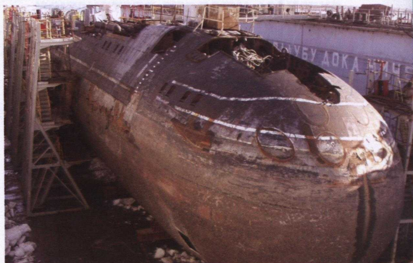
Nuclear submarine in floating dry dock prior to dismantling
