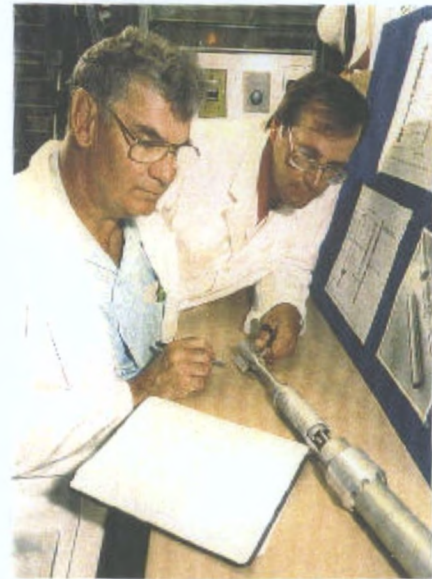
"Final Inspection of the Specimen Capsule Assembly of the Uniaxial Creep Insert for a MK-IV FN Rod"
