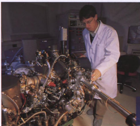
AECL's Secondary Ion Mass Spectrometer (SIMS).
