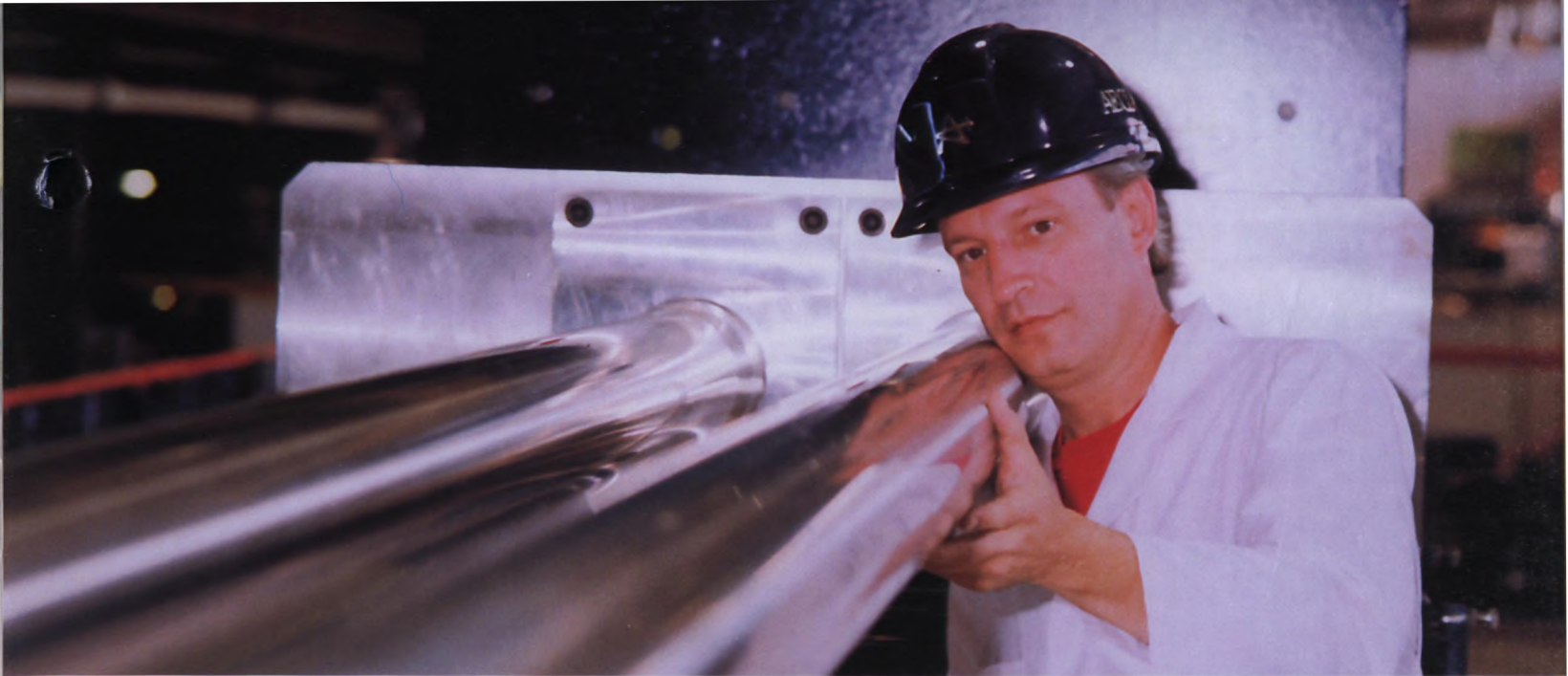
The CNF will supply the conditions to test full-diameter CANDU pressure tubes in conditions of controlled chemistry, temperature and pressure.
