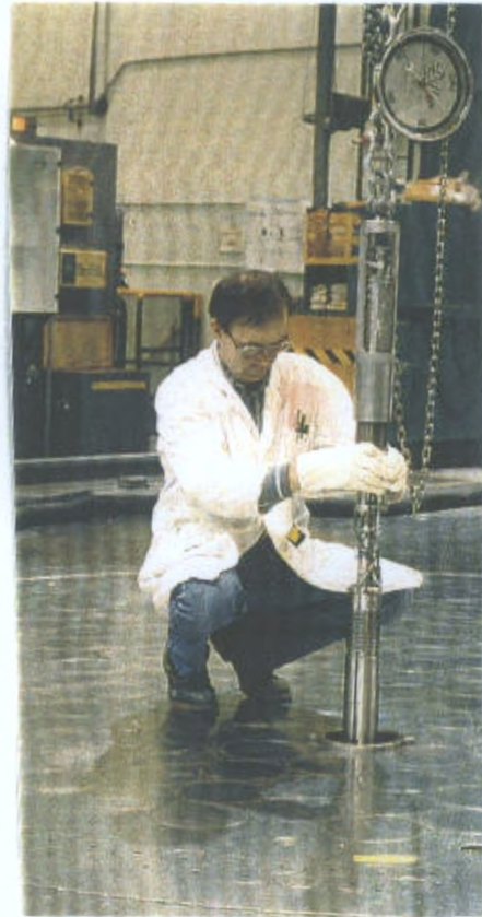
"Installing the BTF Fuel Test Assembly"
