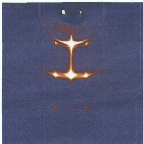
Diffraction pattern from aligned, fully hydrated lipid multibilayers in the ripple, P_B , phase hydrated from water vapour.
