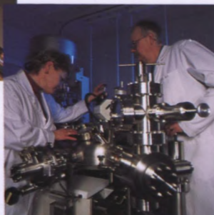
Specimen undergoing X-Ray Photoelectron Spectroscopy (XPS).
