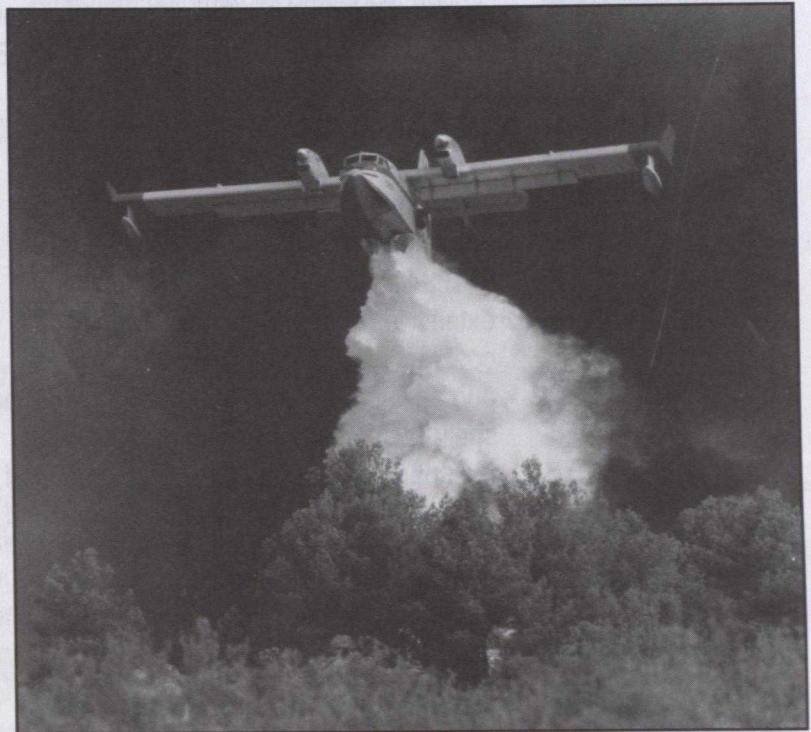
The CL-215 aerial firefighter, built by Bombardier Aerospace. Photo courtesy of Bombardier Aerospace
