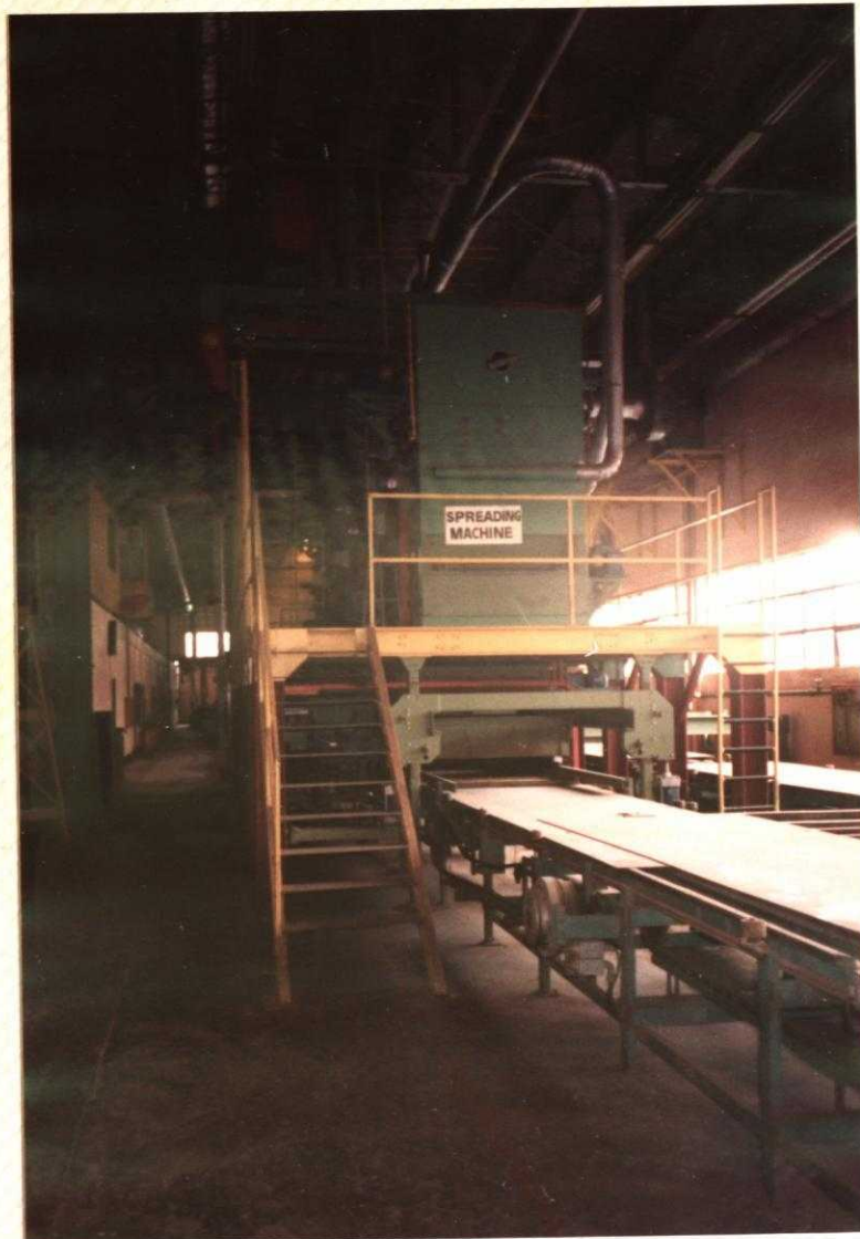
No. 17. OSB Panel assembly line with spreading machine in foreground.
