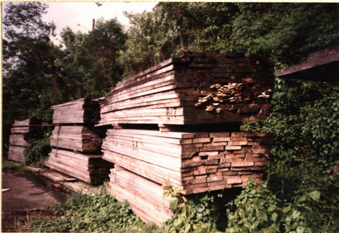
No. 28. An example of wastage through neglectful handling of lumber not piled on stickers.
