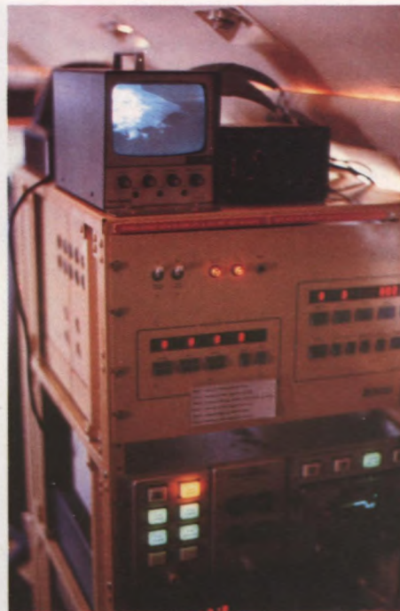
ALICE, Knudsen Engineering's high-performance image enhancement and display system for airborne remote sensing, is used for oil spill reconnaissance, search and rescue, and many land applications.
