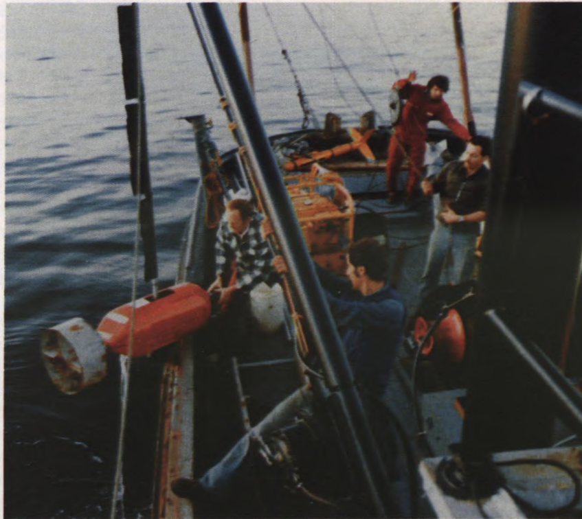
A McElhanney crew retrieves a narrow beam sounding fish.
