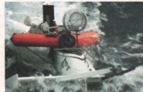
Guildline's Batfish is a programmable towed body which can be "flown" at a static depth or automatically in a sawtooth pattern for rapid gathering of oceanographic data.
