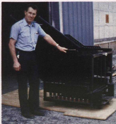
Eastern Marine's multiple net zooplankton sampler, ready for electronics to be mounted.
