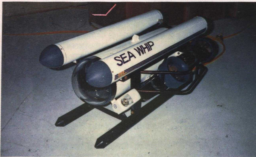
The Sea Whip, made by Sea Scan Technology, is a heavy-duty, low-cost remotely operated vehicle (ROV) which operates to 366 metres.
