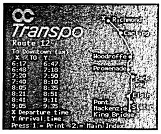
VAST allows a customer to graphically create, store, recall and telecommunicate videotex graphic frames. It includes features such as NAPLPS graphic frame creation, local storage on diskette or mass storage, sequential, menu-driven, or automatic sequence framepresentation routines as well as the capacity to access and transmit frames to and from other computer sources.
