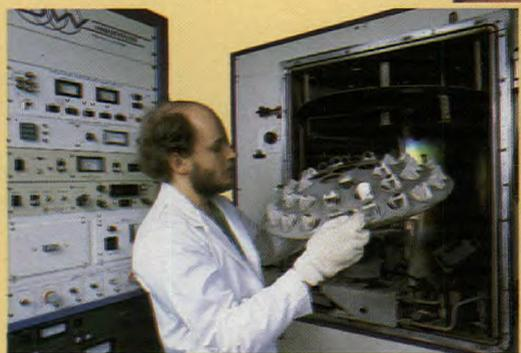
*Design, development and application of multilayer thin film coatings for UV, visible and IR materials.*
