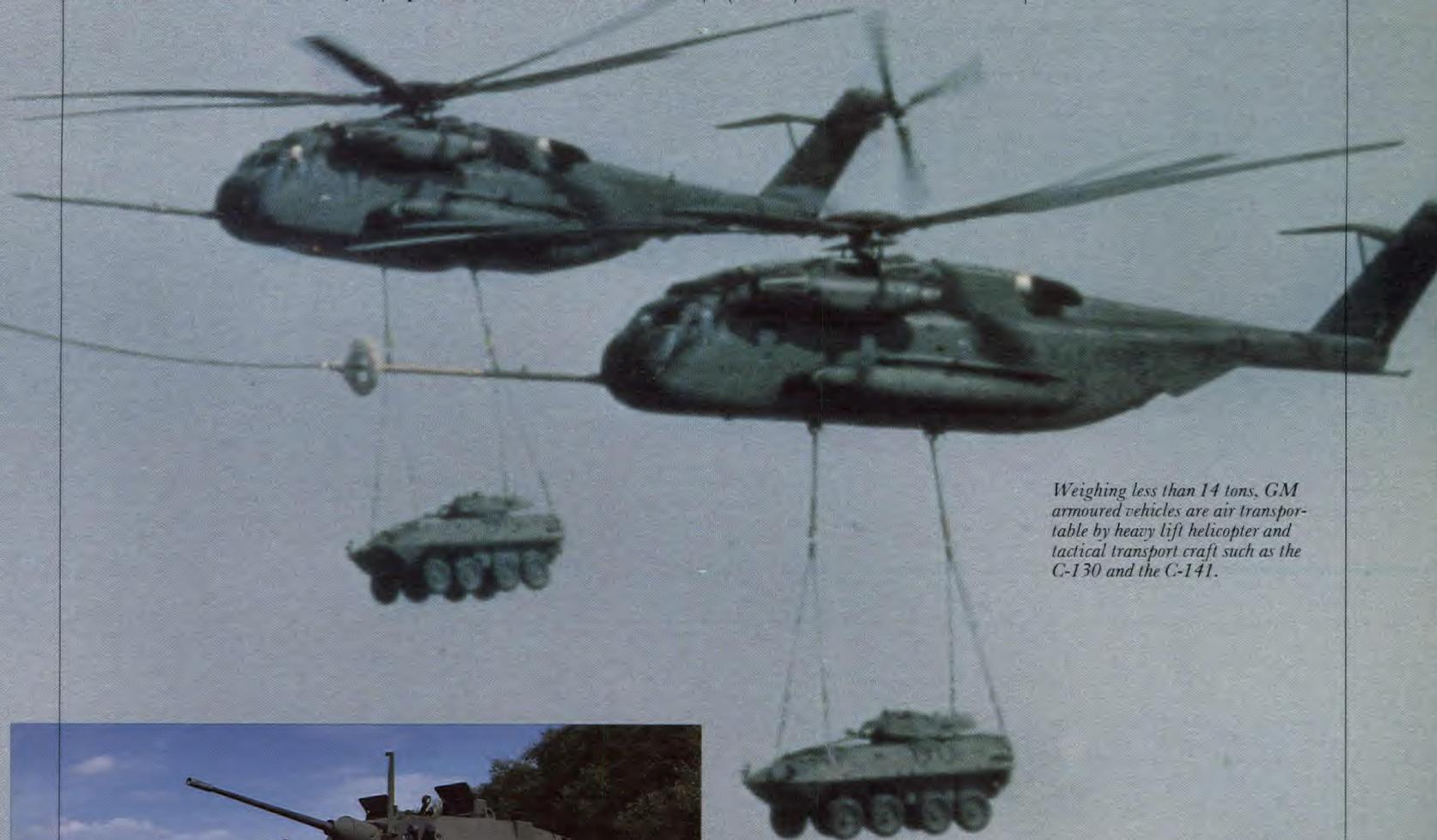
*Weighing less than 14 tons, GM armoured vehicles are air transportable by heavy lift helicopter and tactical transport craft such as the C-130 and the C-141.*
