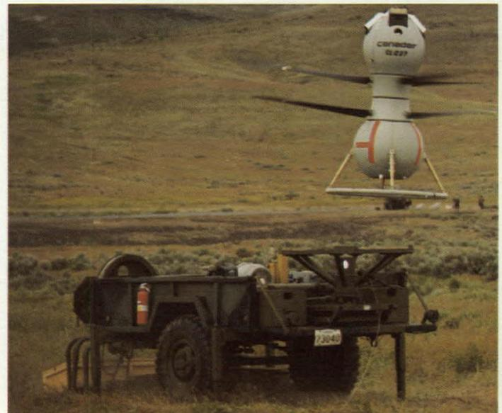
*CL-227 Sentinel unmanned surveillance and target acquisition system.*
