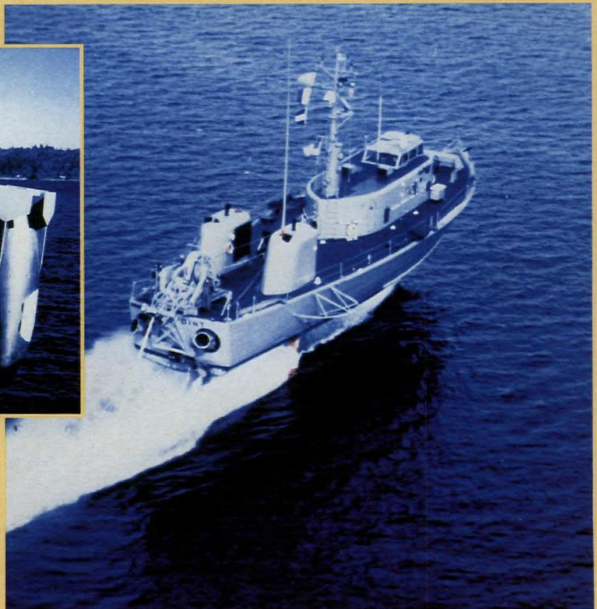
*HS-1001 VDS system on high-speed trials on USN PCH-1 High Point.*
