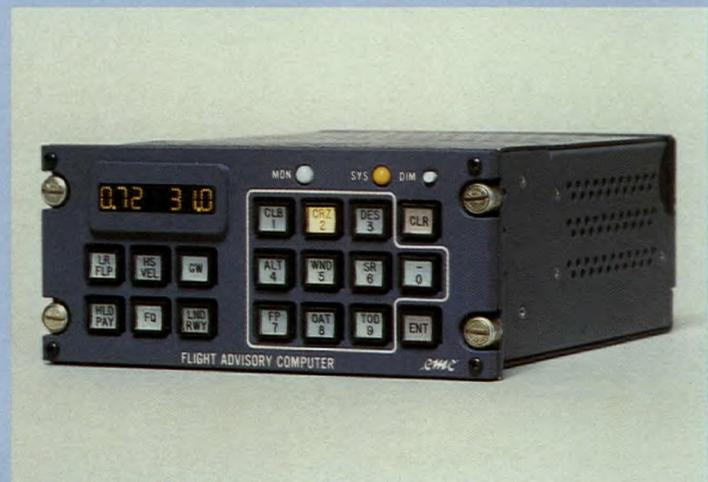
optimum/safe operating advisories to the crew. The FAC serves as an electronic flight manual that provides direct readouts for operation of the helicopter in response to flight condition inputs by the crew.
