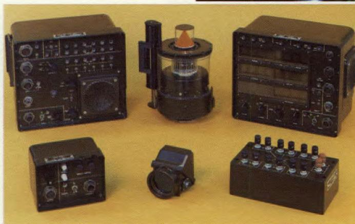
*The artillery gun alignment and control system (GACS) is three systems in one — a rapid automatic north alignment system for all guns, a digital fire order transmission system, and a two-way voice communication system.*
