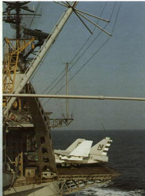
*Elevator hoisting aircraft from below deck storage. Elevator wire rope from Greening Donald is used to hoist elevator.*
