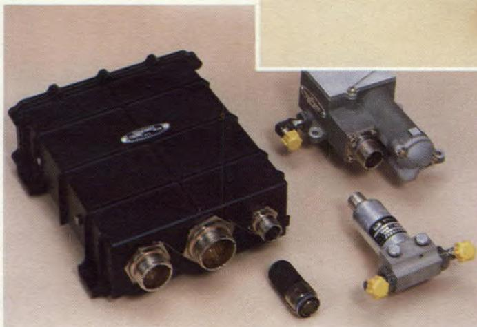
*The PT6A-62 electronic limiting system limits and monitors critical engine variables. Designed for high-performance turbo-prop trainers, the device allows single-lever control similar to a jet aircraft, and maintains constant engine power during aerobatic manoeuvres.*
