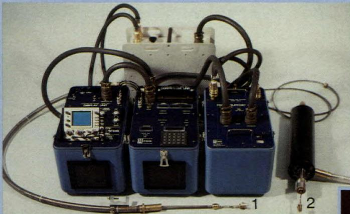
*The NDE-2 automatic tube analyzer showing superheater (1) and generator (2) probes with support modules.*
