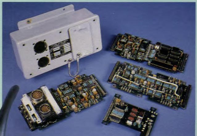
*Steering control, hydraulic and electronic control units.*
