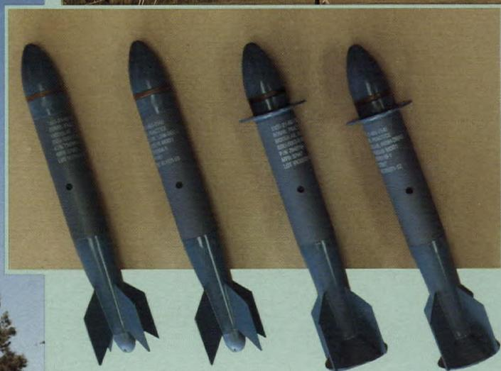
*Modular practice bombs are available in high and low drag configurations. Weighing only 2.83 kg (6.25 pounds), these bombs are adaptable for use on most of today's modern fighter aircraft.*
