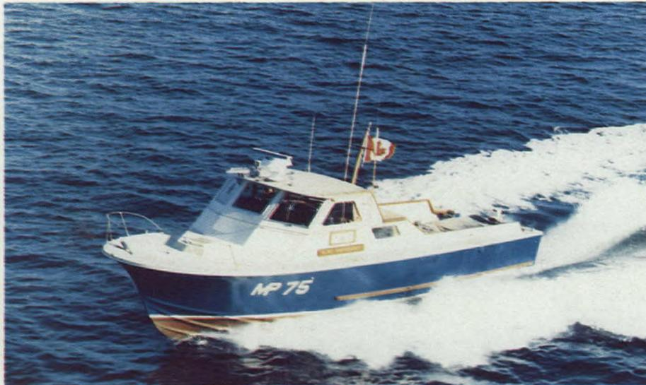
*The 12.5-metre Canoe Cove / R.C.M.P. patrol vessel with 4.5-metre beam is powered by twin 250-hp Caterpillar diesels (187.5 kW). Service speed is 24 knots and top speed, 25 knots.*
