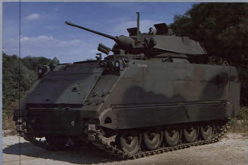
*The useful service life of M113 inventories can be extended with GM enhancements such as Delco 25-mm (1-inch) turret integration to meet modern firepower standards.*
