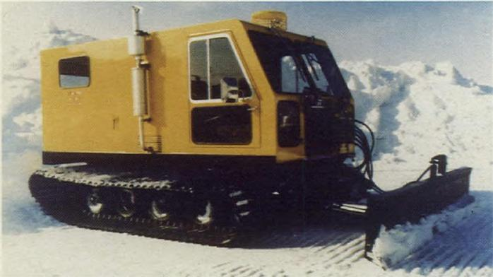
*"SKIDOZER" personnel carrier equipped with hydraulic snow plow.*
