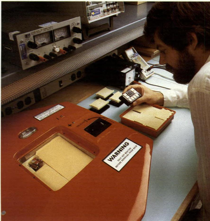
*Pre-production solid-state memory modules are flight-tested in this deployable crash position indicator air-foil that ensures the survivability of flight data.*
