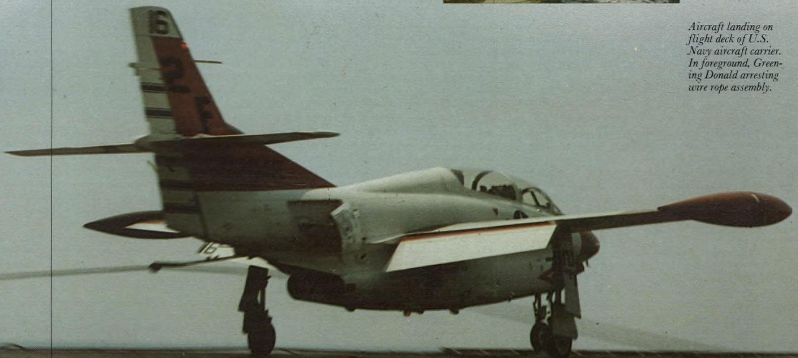
*Aircraft landing on flight deck of U.S. Navy aircraft carrier. In foreground, Greening Donald arresting wire rope assembly.*
