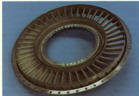
*J85-CAN-40 turbine nozzle produced by Orenda is typical of the extensive range of spares manufactured for the J79 and J85 engines.*
