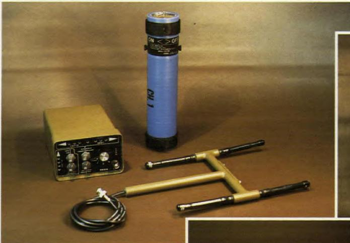
Military parachute tracking system showing a parachute transmitter (blue) and direction finding receiver with detachable D/F antenna.
