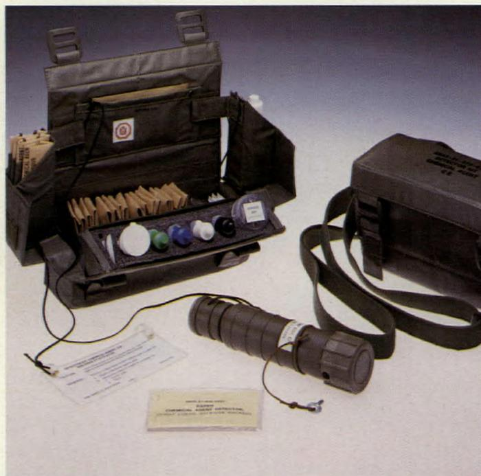
2. pressing the detector body into the holder so that the test papers are in contact. The test paper will turn blue or green in the absence of nerve agent vapour. If such vapour is present or the test has been incorrectly performed, the test paper colour will remain unchanged.
