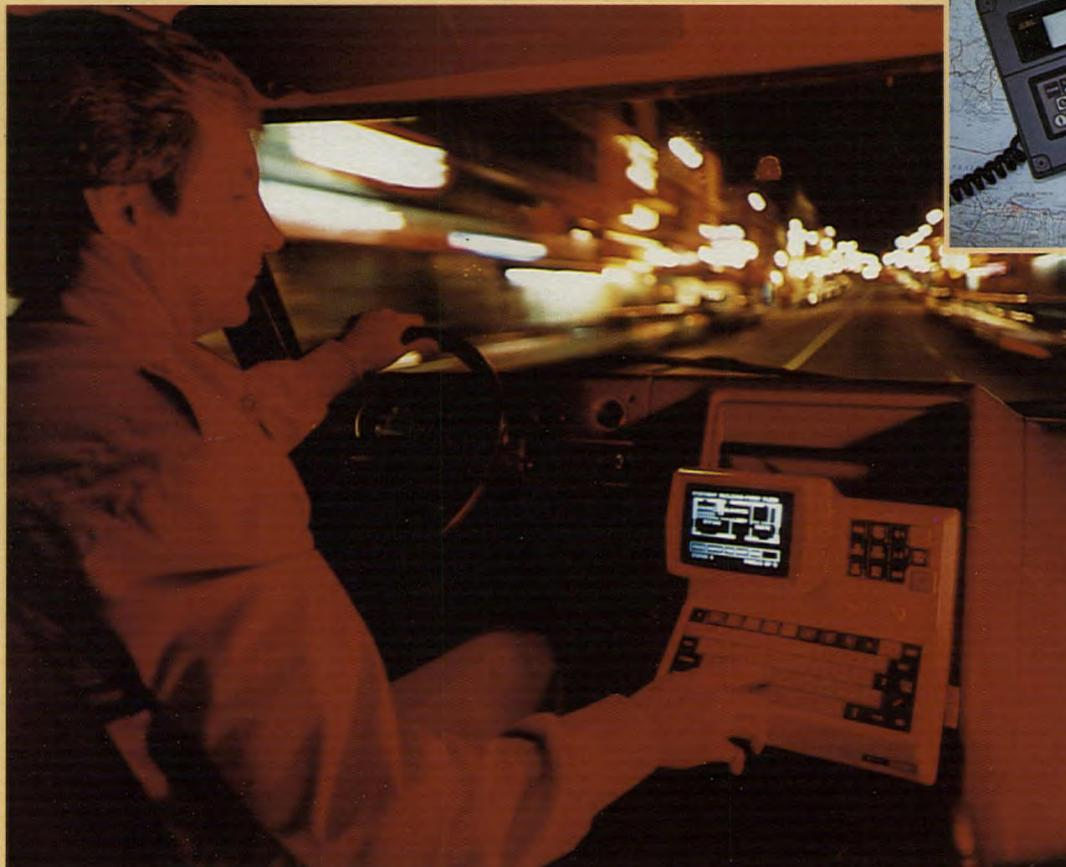
*Tactical data terminal connects directly to AN/PRC-77 radio.*
