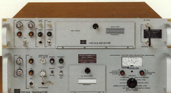
◀ Air traffic control receiver and transmitter.
