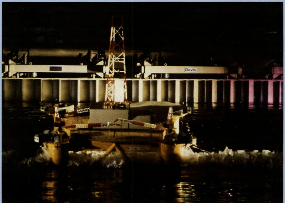
*Example of wave-making machines used for testing semi-submersibles.*
