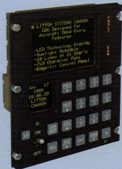
*The Litton-built control display unit features two LED displays on one piece of avionics equipment.*
