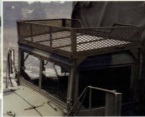
*Roof rack on 2½-ton cargo truck.*
