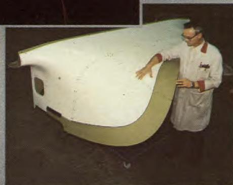
*Inspection of a wing to fuselage fairing composite for the DASH 8 aircraft.*
