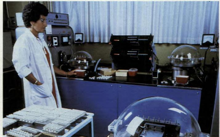
*Automatic sealing station for glass encapsulated crystals.*
