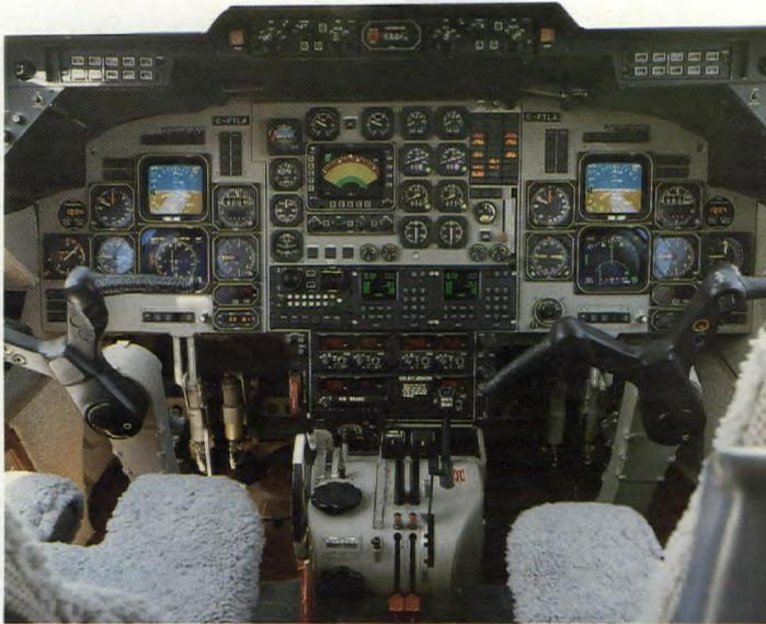
*Avionics systems design and integration has been an Innotech strength since 1955. Shown here is an all-digital 5-Tube EFIS (electronic flight instrument system) avionics package in a business jet.*
