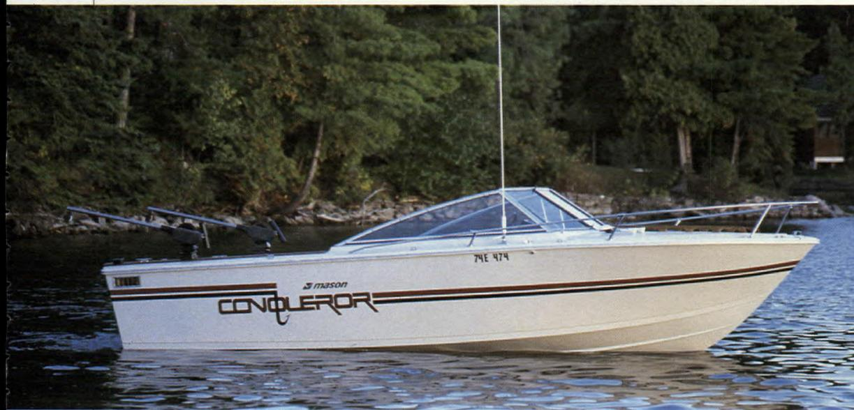
Designers and builders of reliable top-quality boats since 1867, Mason manufactures a variety of vessels with 100-per-cent hand-laid-up fibreglass hulls. Mason boats range from the 5-metre (17-foot) CCF17-Centre Console Fisherman, with the unsinkable cathedral hull, to the 6.7-metre (22-foot) CF220-Cuddy Fisherman, CC238-Cuddy Cruiser and 8-metre (27-foot) MX284-Cabin Cruiser with their deep vee hulls.
