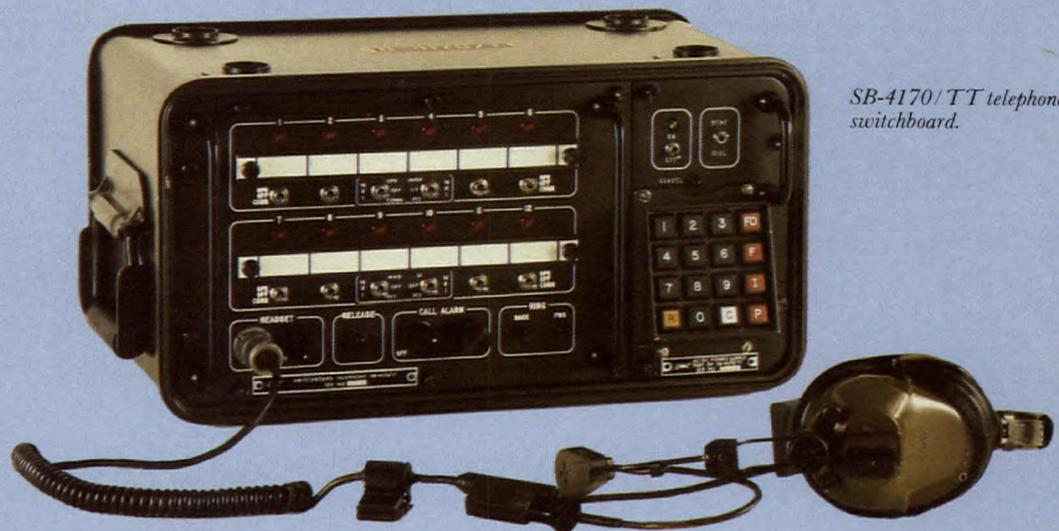
*SB-4170/TT telephone switchboard.*
