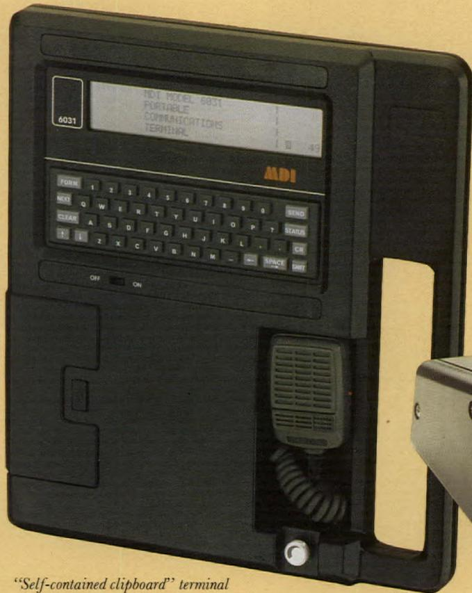
*"Self-contained clipboard" terminal with voice option and built-in 800-MHz radio.*
