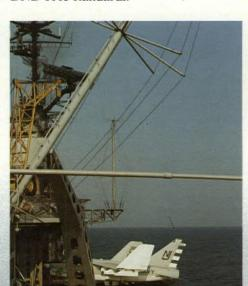
Elevator hoisting aircraft from below deck storage. Elevator wire rope from Greening Donald is used to hoist elevator.
