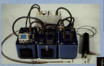
The NDE-2 automatic tube analyzer showing superheater (1) and generator (2) probes with support modules.
