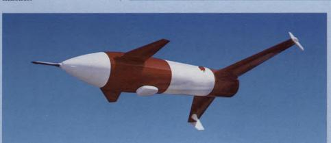
Robot-X. A manoeuvrable low altitude target.
