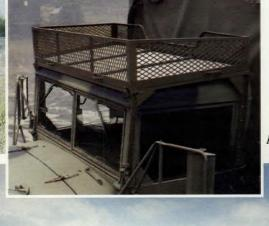
Roof rack on 21/2-ton cargo truck.
