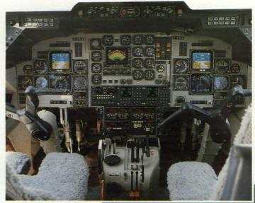
Avionics systems design and integration has been an Innotech strength since 1955. Shown here is an all-digital 5-Tube EFIS (electronic flight instrument system) avionics package in a business jet.
