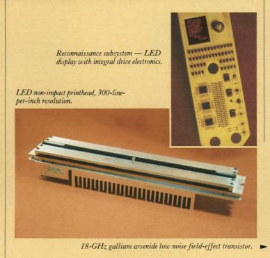
Since incorporation in 1977, Optotek's opto-electronic semiconductor products have enjoyed widespread international acceptance in the military, avionic and industrial sectors. The company's vertically integrated product capability encompasses lightemitting diode displays and associated electronic subsystems; infrared photodetectors; and gallium arse-
