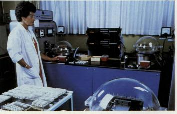
Automatic sealing station for glass encapsulated crystals.
