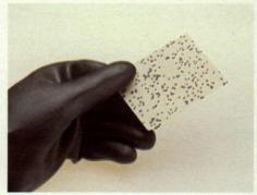
Paper chemical agent liquid detector following exposure to liquid chemical agent spray — 3-Way liquid adhesive backed.
