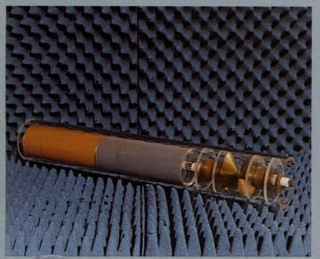
Mock-up of an expendable microwave jammer developed by Tele nus.
