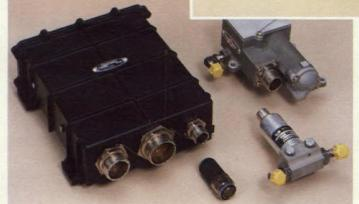
The PT6A-62 electronic limiting system limits and monitors critical engine variables. Designed for high-performance turbo-prop trainers, the device allows single-lever control similar to a jet aircraft, and maintains constant engine power during aerobatic manoeuwes.
