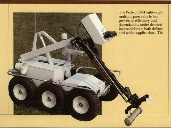
vehicle is designed for the remote handling of improvised explosive devices (IED), surveillance, fire-fighting, handling of radioactive material, anti-hijacking and hostage-taking — and many other varied and related functions.
