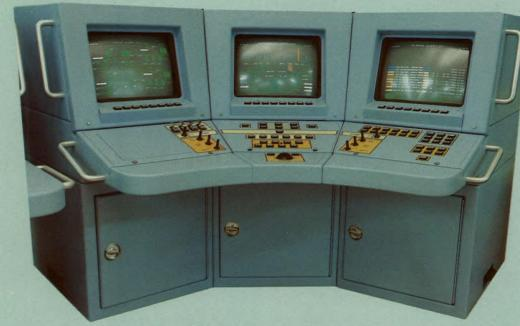
Integrated machinery control system for the Canadian Forces' new patrol frigates is manufactured by CAE Electronics Ltd.
