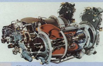
PT6 turboshaft, as a TwinPac®, is used in the Bell AH-17 and T gunships, the UH-1N and CUH-1N transport helicopters, and ASW helicopters built by Agusta. As a single engine, two are installed in Sikorsky's S-76B.
