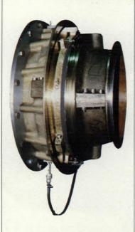
Tyton test rig for main propulsion shaft seals.
