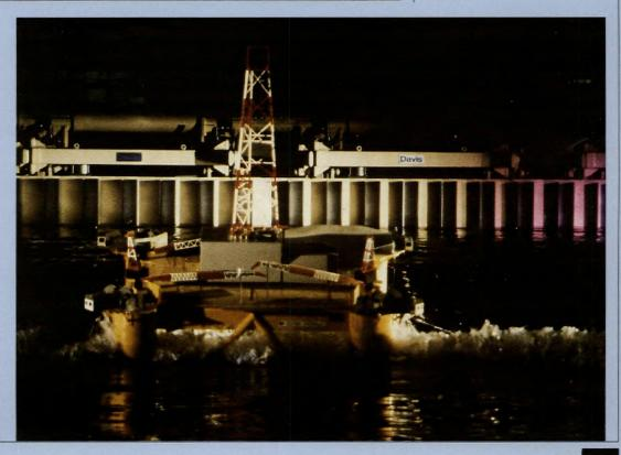
Example of wave-making machines used for testing semi-submersibles.
