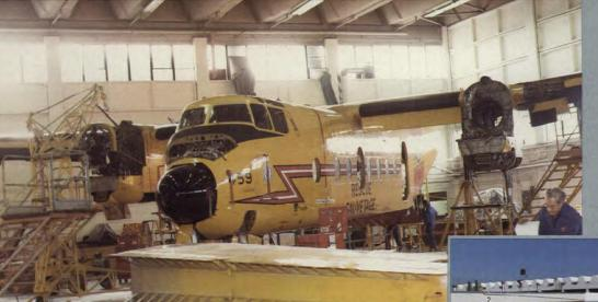
Canadian Forces Buffalo aircraft undergoing a repair and overhaul program at Field Aviation West Ltd.
