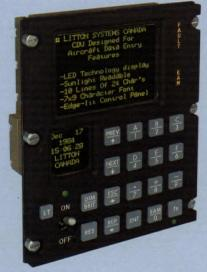
The Litton-built control display unit features two LED displays on one piece of avionic equipment.
