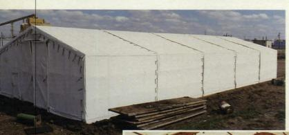
Norseman Shelters manufactures portable buildings made with a steel frame and fabric cover and designed for fast, easy erection by unskilled personnel. Norseman's pin and pocket assembly system requires no bolts, allows personnel to keep their gloves on, and eliminates the need for special tools. The frame and fabric dismantle into easy-
