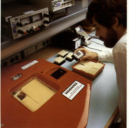
Leigh's TACAN beacon transponder features rapid channel selection and remote maintenance monitoring
