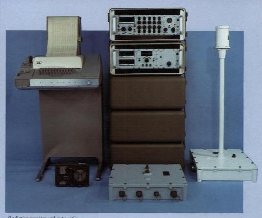
Radiation monitor and automatic alarm system AN/GDQ-3.
