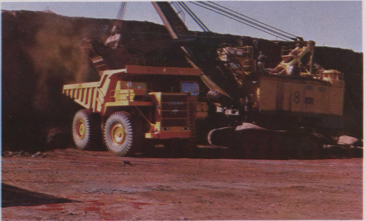
*One of the Unitrig 36 electric haul 154.2 tonne payload trucks in use at one of the Hammersley Mines.*
