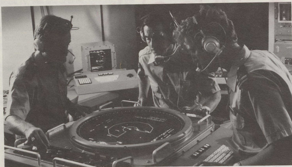
The situation information display of Litton's automatic data link plotting system that can be adapted for use on ships of various classes.
