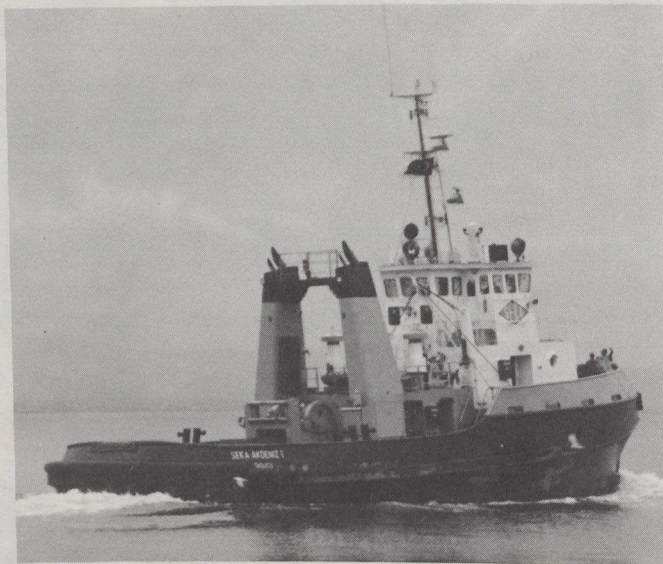
Tug built for Turkish coastal forest industry is powered by two 850-horsepower engines and carries a crew of nine.
