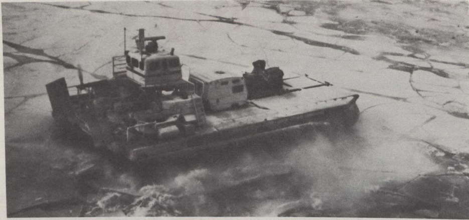
NRC scientists are studying air-cushion vehicles to determine why they can break ice more easily and economically than conventional icebreakers. Air-cushion vehicles were developed mainly for carrying cargo over rough terrain.
