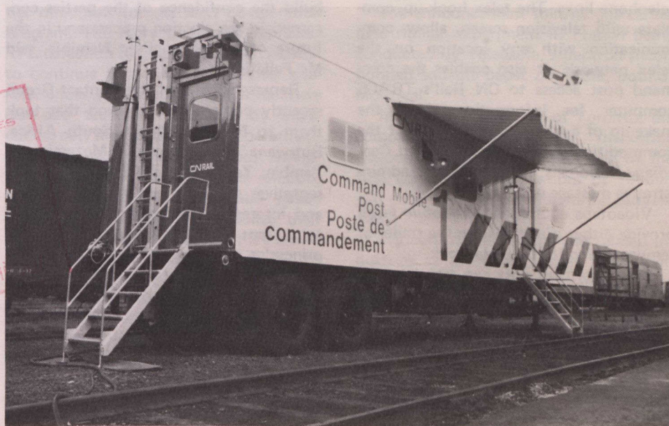
This special communications trailer was custom-built by CN Rail at a cost of some $250,000. Designed to be the Command Post at the site of a major derailment, Mobile 1 can travel by highway and rail flat-car.
