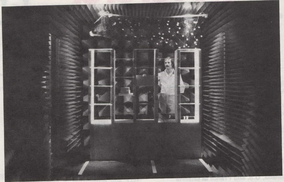
This specially constructed chamber at the National Research Council in Ottawa has been designed to determine safe exposure levels of microwave radiation on animal tissue. The project will assist government in establishing realistic safety standards for such common sources as radio transmitters, radar and domestic microwave ovens.
