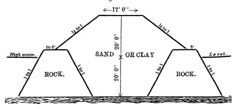
Rock sides, earth core and top cost per lineal foot......\$100 25
