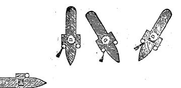
If A sees a White Mast-head Light above the Green Light, A knows that the vessel is a steam-vessel, and is either approaching her in the same direction as B, or is crossing to starboard in some direction, as D D D.
