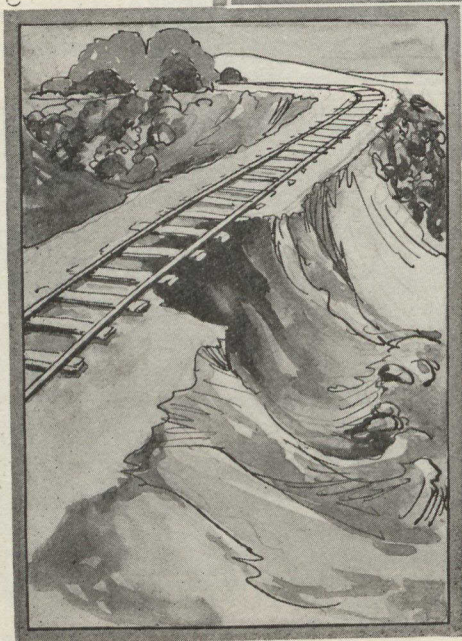
Showing how foundations often slide from under tracks.
