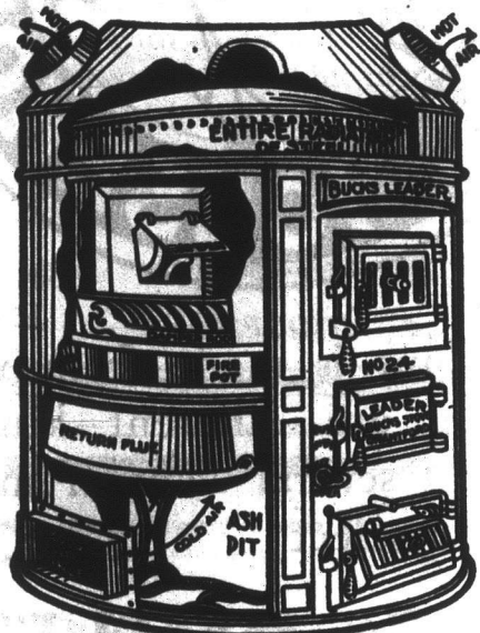
Sectional View of Buck's Leader Furnace
