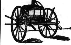
No. 1 and 2, with horse-drawn cart, can be used on orchards, vines, row crops or weeds. As shown here it is arranged for row crops and weeds, but separate attachments adapt it to other uses. Adjustable width of track and rows, all-brass Spramotor, brass ball valves, automatic agitator and compensating plunger. High grade throughout. For one horse only. Price \$47 to \$54
