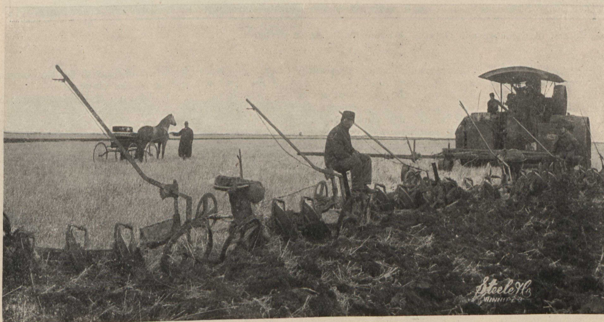
When Man Begins His Work—Steam Ploughs are much used in the West, where they do Ploughing on Contract at about $3.25 an acre. The Average day's work for an Engine is 20 acres
