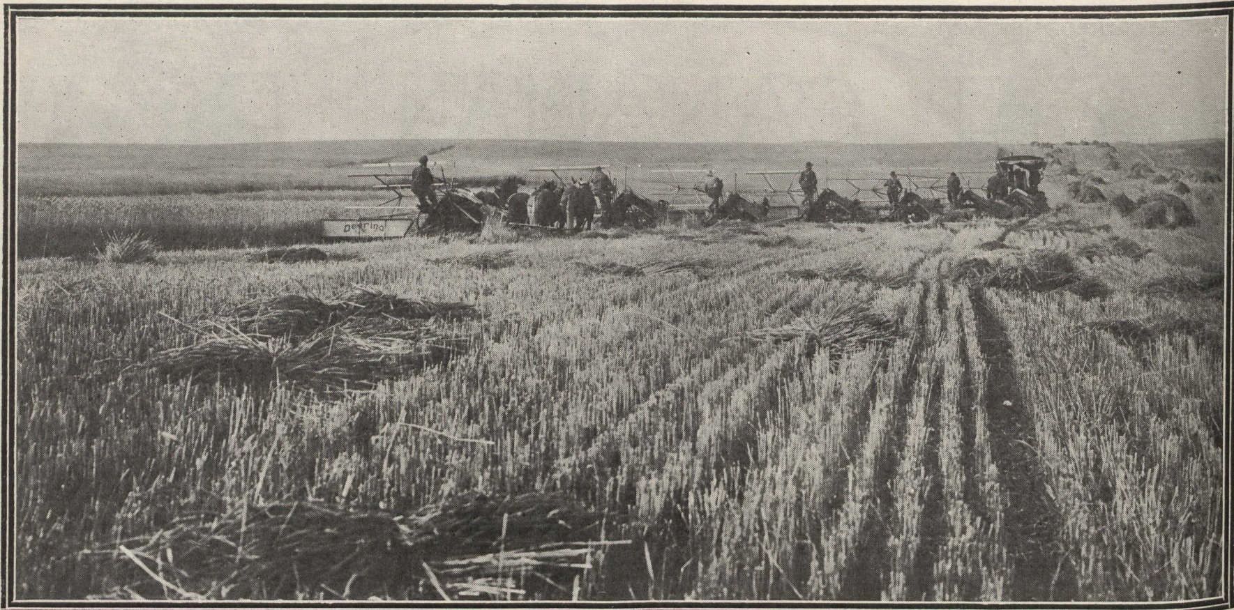
Six binders drawn by a "caterpillar" engine did the harvesting this year on the 4,160-acre Crowfoot Farm in Southern Alberta. The six binders mowed down the crop in a 48-foot swath. The cost of the binders and engine alone would be equal to the value of a good crop on a fair-sized farm.
