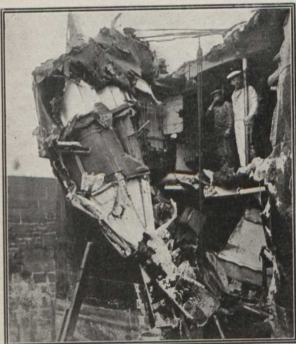
The Hole in the Side of the Destroyer "Jackal," Made When She Failed to Clear the Bow of the "Thunderer" Off Tay Mouth Recently. The Steel Plates Crumpled Like Paper, But Fortunately No Lives Were Lost.
