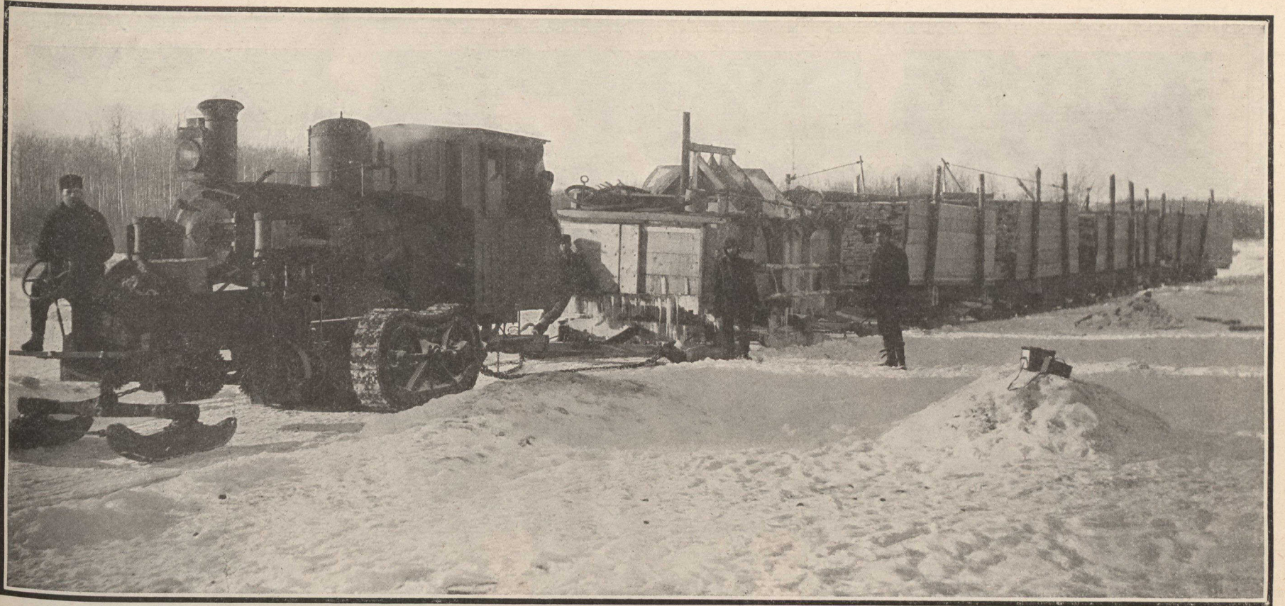
A Snow Locomotive which draws Logs to the Sturgeon Lake Lumber Company's Mills, not far from Prince Albert, and draws Lumber from the Mills to Prince Albert. It will draw 100,000 feet at one load.
