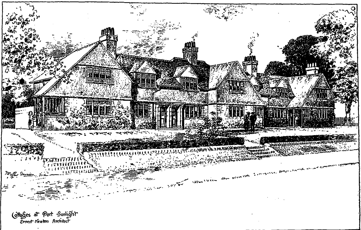
Cottages at Port Sunlight. An Eminently Successful Group Containing Seven Houses in Which the Plan of the Interior is Identical in Every Case. The Irregularity of the Frontage and Skylin: Lends a Pleasing Element of Variety, While the Two Entrance Porches Side by Side in the Projecting Bays Further Contribute this Way in Addition to Effecting Considerable Economy in Floor Space. Ernest Newton, F.R.I.B.A., Architect.
