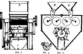
from coming in contact with the wire, and only the lighter particles are carried over the top edges of the protectors. Air is permitted to enter the machine at i through the hoppers II. Aside from this, air may be permitted by means of the adjustable valve m; tt are self-acting valves for the purpose of delivering the ground stock to the outlet of the hopper. Alilling.
