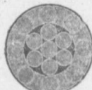
Locked Coil Aerial Cable or Colliery Guide.
