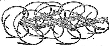
(FOLDED FOR SHIPMENT OR STORAGE.) Fluted Steel Frame of Great Strength; Spring Steel Teeth (Tempered\_in Oil); Malleable Hinges.
