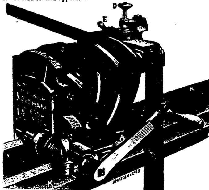
The card when being mounted is taken from the skip and passed through the trough *D* to the drum *A*, around which it passes over the three divisions to the tension lever and on to the cylinder *F*, the tension being regulated by the screw on the weight in the trough *D*, or by the brake on the drum shaft, and the card is mounted by turning the handle *R*. The tension arrangement is as follows: The
