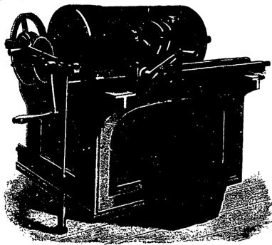
The double-purchase jack U is fixed on the cylinder, or doffer shaft, and is secured thereto by a screw and die which increases its hold on the shaft as the tension on the card fillet is increased; it is fitted with chain and change wheels for working the machine, which is actuated by the handle R. The rest and tool X is used for turning-up wood rollers or cylinders, and is fixed on the bed K in place of the card tension apparatus.
