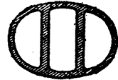
Oval Traps.—Fig. 5.—Horizontal Section Through A B of Traps shown in Figs. 3 and 4.
