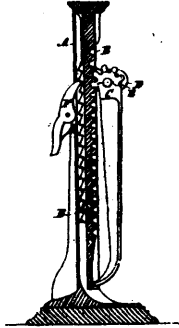
3891 Scott's Carriage Lifting Jack.
