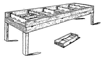
inches higher than the lower end. The water which runs out from the last compartment is prevented running out the whole width of the case by means of two pieces of wood, which are fastened to the sides, and reach nearly to the middle, and is carried off by a pipe.
