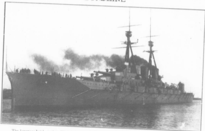
The Japanese battle-cruiser "Kongo", a vessel of 28,000 tons and 28 knots, armed with eight 14-inch and sixteen 6-inch guns. The "Kongo" is the most powerful ship of her class in the world. Courtesy Montreal "Star."
