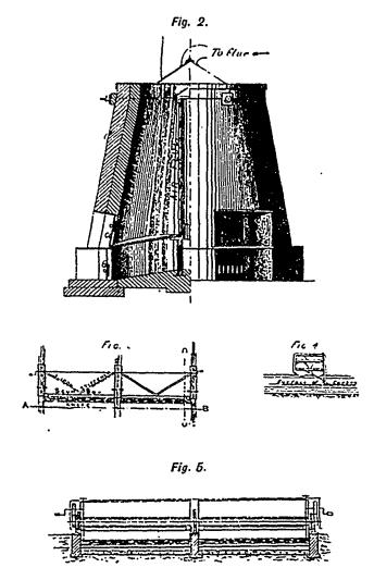
Fig. 1—Detail of filter beds, showing formation of beds. Fig. 2—Sectiona elevation of carbonizer. Fig. 3—Plan of Scum plow. Fig. 4—Sectional elevation at C, D. Fig 5—Sectional elevation at A, B.
