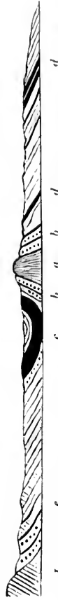
Fig. 40.—Ideal section representing the present arrangement of the Coal formation of Southern Pictou, Nova Scotia. a , Devonian ridge; b , conglomerate; c , great Coal measures; d , minor Coal measures; e , Lower Carboniferous; f , Silurian.
