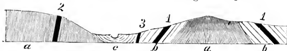
Fig. 160.—Ideal Section, showing the general relations of the Iron Ores of the East River of Pictou. 1. Great bed of Red Hematite. 2. Vein of Specular Iron. 3. Vein of Limonite. (a) Older Slate and Quartzite series, with Felsite and Ash Rocks, etc. (b) Lower Helderberg formation and other Silurian Rocks. (c) Lower Carboniferous of the East Branch of East River.
