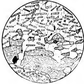
Figure 6.—Sillimanite-Gneiss, west shore of Trembling Lake. Sillimanite, Quartz, Orthoclase, Biotite and Pyrite. \times 38 .
