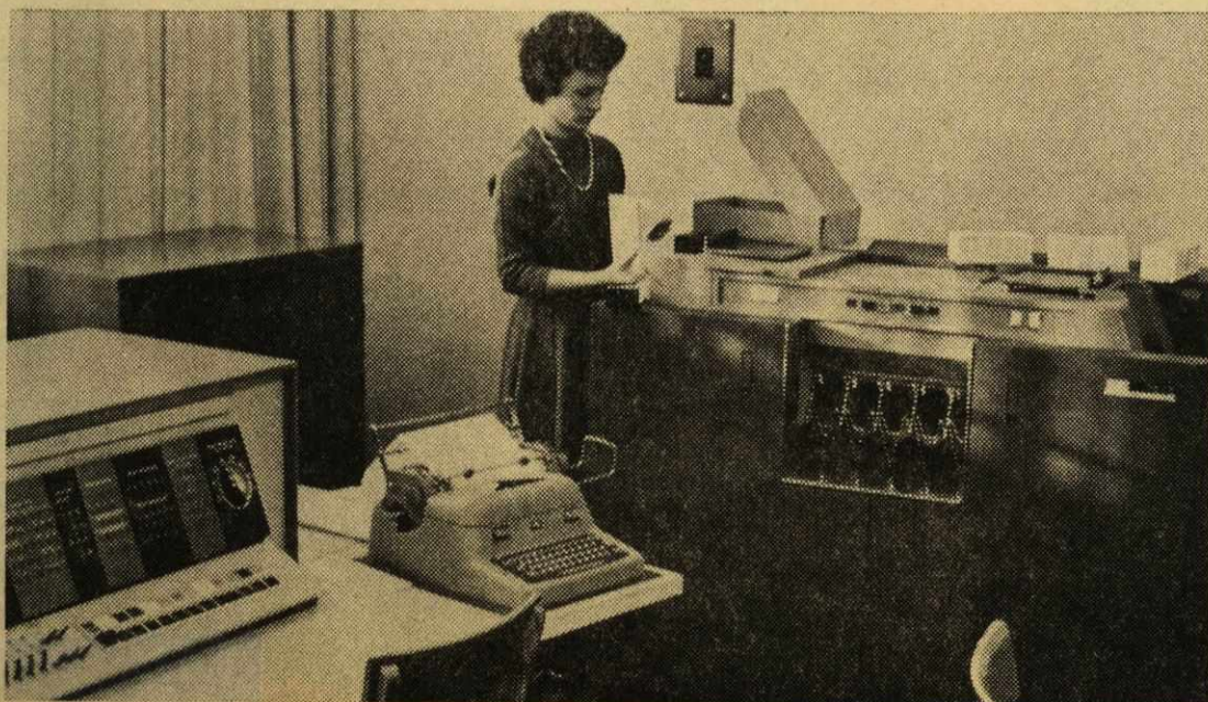
MISS JUDITH HUNTER operates the IBM 1622 read-punch unit. Computer with typewriter is at left.
