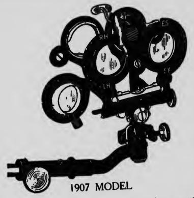
The "Universal" combines in one instrument a 3 cell trial frame with patent revolving cylinder cells; I Risely Rotary Prism; I Multipe Maddox Muscle test; I Stevens' Phorometer.
