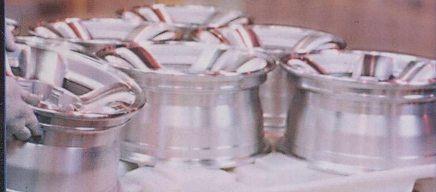
The plant produces aluminum-alloy wheels from British Columbia aluminum using low-pressure diecasting technology.
