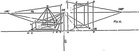
base; complete the square; at f erect a perpendicular equal in height to the side of the cube (5'), and from its upper extremity draw a line to CV; but this line is in the HL, therefore the top of the cube is on a level with the eye, and will appear as a straight line; from the corners of the base erect perpendiculars to meet HL.
