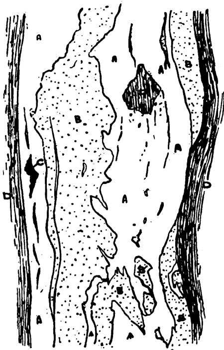
A, quartz (granular); B, blende; C, galena; D, argillite. Scale half full size.
