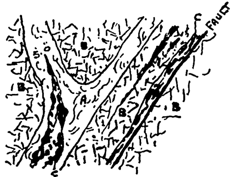
A, argillite, crushed and crumpled, and bedding partly obliterated; B, felspar porphyry; C, galena and blende. Scale 8 ft. to an inch.
