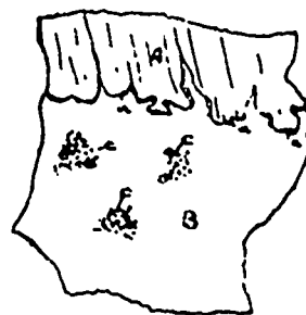
A, siderite, altered to limonite at edge a; B, galena (granular); C, tetrahedrite. Scale full size.
