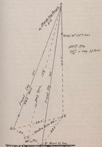
Fig. 2.—Isometric Sketch Showing Deduced Dimensions of Shear-legs.
