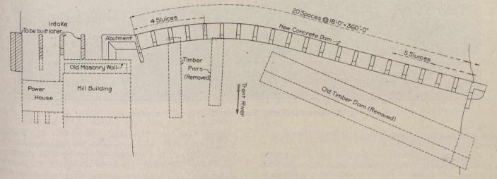
Fig. 1.-Plan of Concrete Dam Across Trent River.
