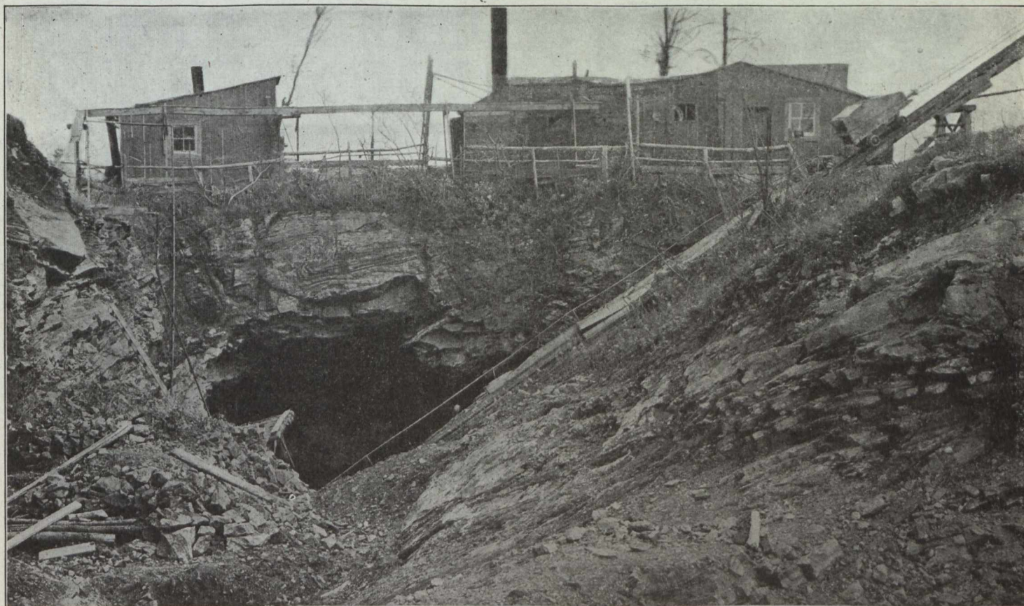
Open cut above workings of Globe Graphite Mining and Refining Company, concession VI, lot 21, township of North Elmsley, Ont. The banding in the limestone is well shown, and a well defined fold is exhibited in the cap rock above the shaft. Graphite bodies tend to occur at the crest of such folds.
