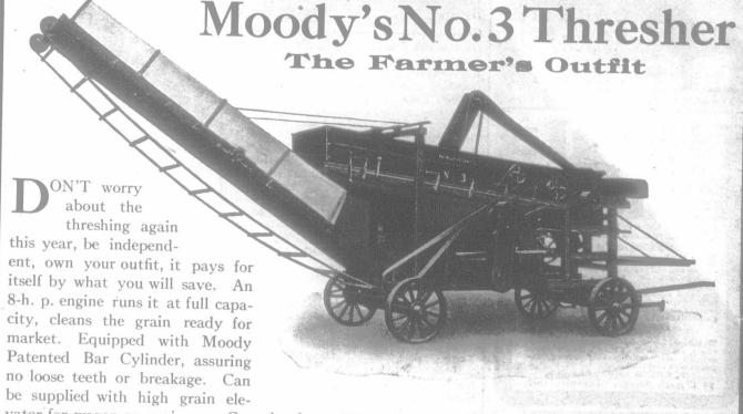
vator for wagon or grainery. Capacity from 600 to 1,000 bushels per day. Handy and easy to operate. Write for price and further particulars.
