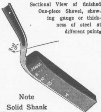
Sectional View of finished One-piece Shovel, showing gauge or thickness of steel at different points
