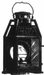
No. 6 Improved Square Tubular Lamp—Outside wick Regulator, Patent Wind Break, 6-in. silvered glass Reflector. Height 16½ in.; width 8½ in.; depth 7½ in.; No. 2 burner, 1-in. wick.
