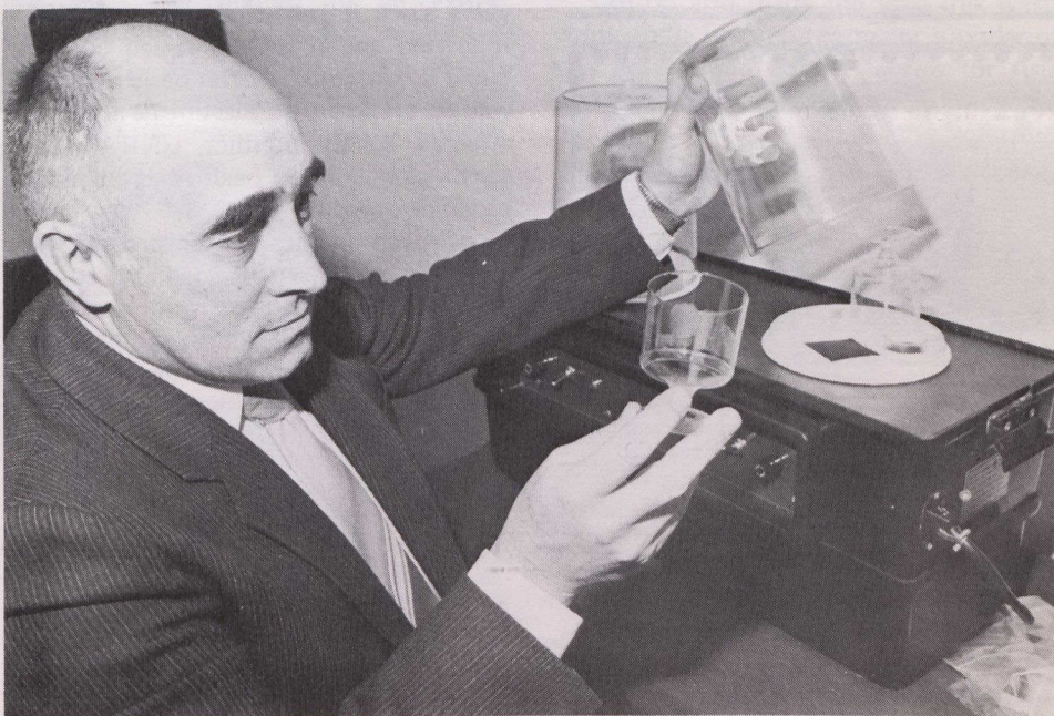
Latent fingerprints soon become visible after Robert Baker, president of Payton Scientific, places a plastic wineglass into the compact Visuprint container which will accomplish its task in ten minutes.
