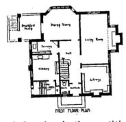
is designed to get as much sunlight as possible and with this end in view every room is placed on the south side, with only corridors, bathrooms, etc., on the north side. One feature
