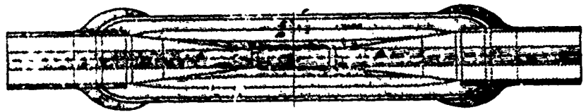
FIG. 3. WASHBURN AND MOEN CABLE JOINT USED.
