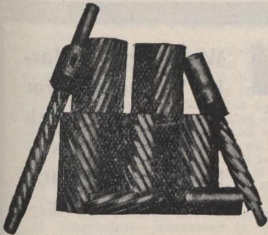
Fig. 1.—Illustrating depth to which cutter teeth may be ground, still retaining their proper hardness.
